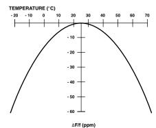
To determine frequency stability, use parabolic curvature (k). For example: What is stability at 45  $^\circ\text{C}?$
